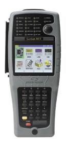
The SunSet MTT ACM+ chassis features a family of Plug-In Modules, providing a wide variety of testing capabilities for the Access Network
